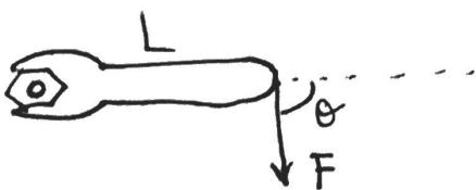
The magnitude of the torque around the bolt is given by:
