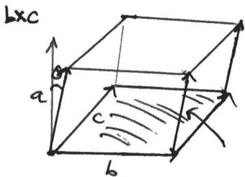
$$\begin{aligned} V &= Ah = \|b \times c\| \cdot \|a\| \cos \theta \\ &= |a \cdot (b \times c)| \end{aligned}$$
