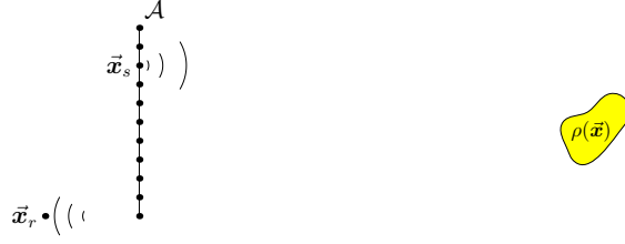
Figure 2.1. Physical setup for array imaging with an array \mathcal{A} of sources \vec{x}_s and a single receiver \vec{x}_r . The scatterer is represented by a compactly supported reflectivity function \rho(\vec{x}) .
