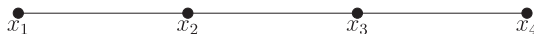
Figure 1. The mass-spring network of Example 2.4 with boundary nodes \mathcal{B} = \{1, 4\} and interior nodes \mathcal{I} = \{2, 3\} .
