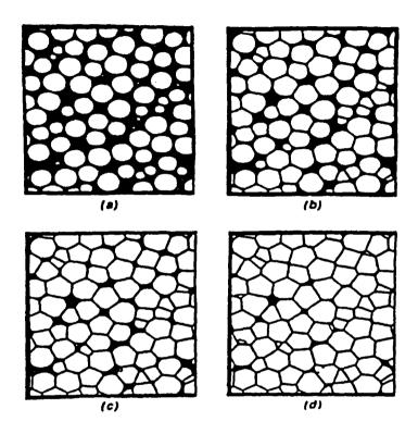
Figure 2: Computer simulation of the consolidation of spherical grains (from [19]), showing decreasing porosity  $\varphi$ , with (a)  $\varphi=0.364$ , (b)  $\varphi=0.200$ , (c)  $\varphi=0.100$  and (d)  $\varphi=0.030$
