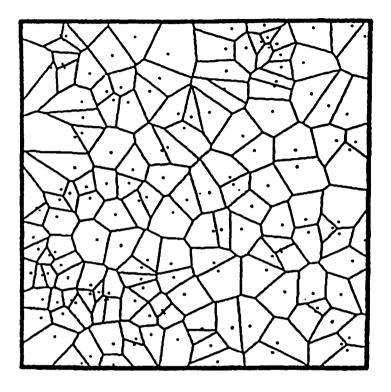
Figure 1: Two dimensional Voronoi tessellation (from [2]). The boundaries of the polygonal grains are formed from points which are equidistant to the dots in two neighboring grains. These boundaries form the channels of easiest flow in consolidated granular media and fractured rocks
