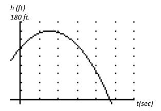
This graph h(t) is the graph of the height of an object in feet at time t. The object has been thrown up in the air from a tall building. The t-axis is in seconds (1 sec per tic) and the h-axis is the distance the object is from the ground in feet. (20 ft per tic)
